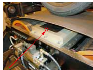
Crack detection sensor
